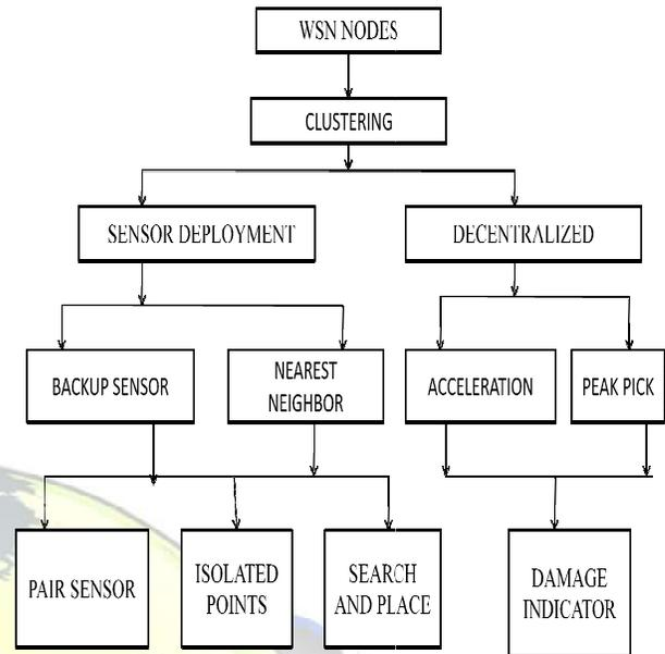
The above figure represents the system architecture to deploy the backup sensors. First, the numbers of nodes are determined. The numbers of nodes are determined depending on the network. It may vary from network to network. When all the nodes are defined along with the base station, the clustering is performed.
