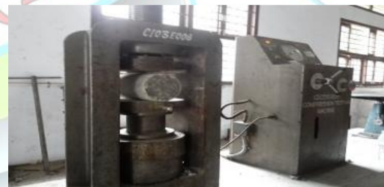
Figure 4: Split Tensile Strength Setup
