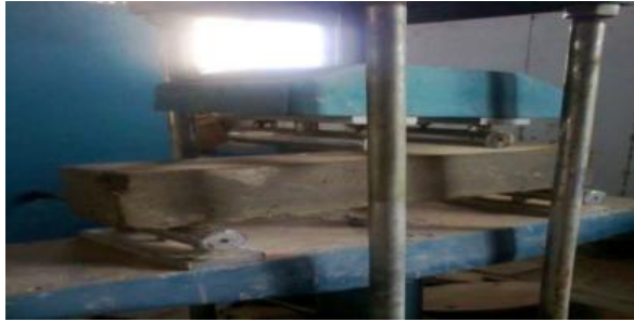
Figure 5: Modulus of Rupture Test Setup
