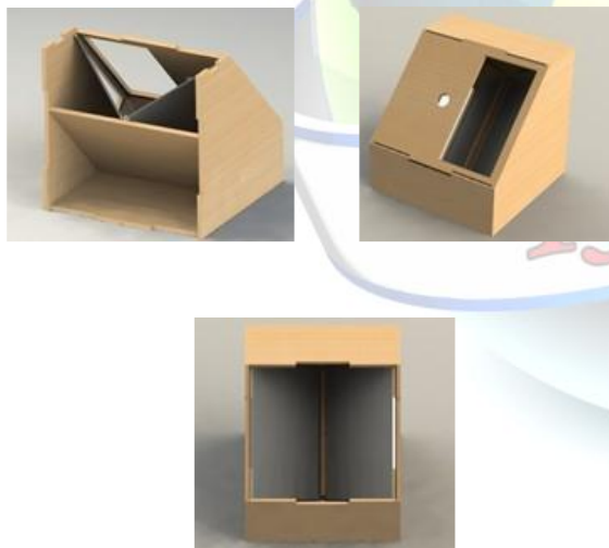
Fig. 2. The mechanical structure of the image capture box. (a) From the back. (b) From the front. (c) Internal structure from the front.[4]
