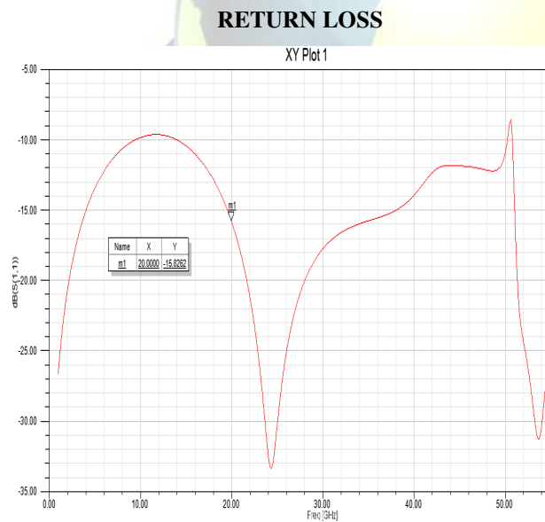
Figure 14: Return loss of loaded ECPW when the switches are on
