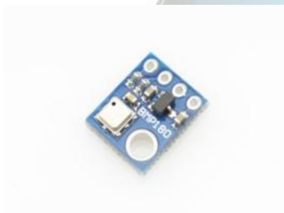
Fig5:BMP180 Pressure Sensor
