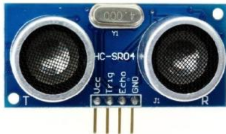
Fig 2. HC-SR04 Ultrasonic Sensor.
