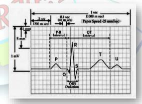
${\bf Figure 1. Typical\ one-cycle\ ECG\ signal\ tracking}$
