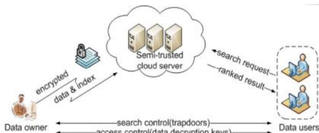
fig.1. architecture of the search over encrypted cloud data.
