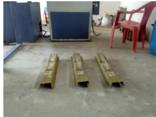
Figure 8 Specimens after flexural test
