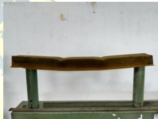
Figure 9 Specimens after flexural test
