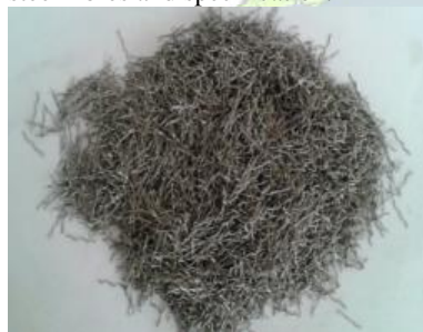
Fig. 2: Round crimped micro steel fibres
