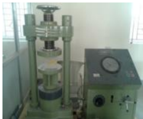
Fig. 3: Testing of cubes
