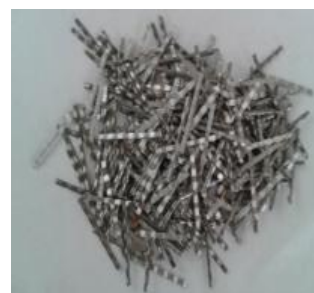
Fig. 1: Flat crimped macro steel fibres
