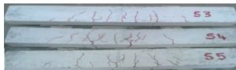
Fig. 13: Failure pattern for all the beams
