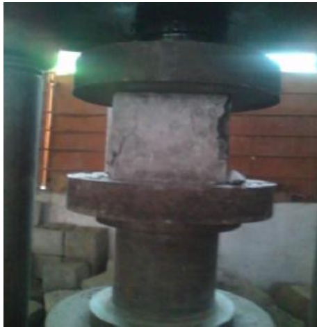
Fig . 2: compressive strength test for specimen cubes
