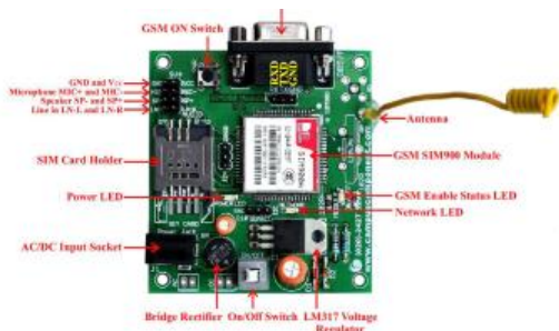
Fig 4.Hardware description of GSM module
