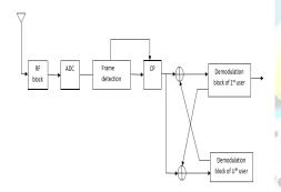
Fig 3. General Receiver Structure for TDMUIC
