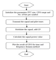
Fig2.Flow of CFO Estimation technique
