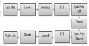
Fig1. OFDMA Block Diagram
