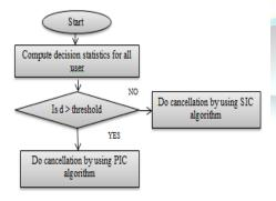
Fig 6. Flow chart for SPIC algorithm
