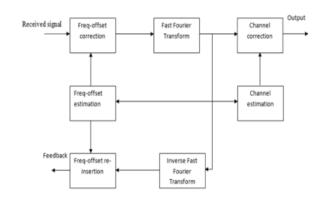
Fig 4. Demodulation Block for SI-MUIC Scheme
