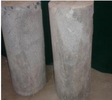
Fig. 18: Failure of Wire mesh specimen
