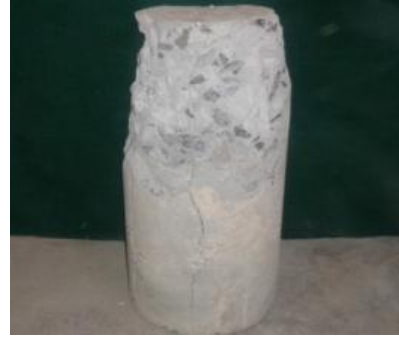
Fig. 20: Failure of Nylon mesh specimen
