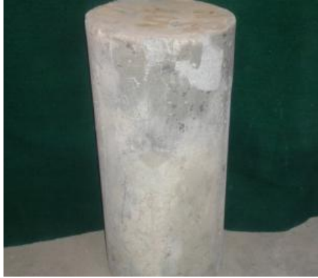
Fig. 17: Failure of glass mesh specimen
