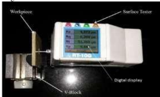
Fig (2): Set up of measuring surface roughness of drilled hole in GFRP by roughness tester
