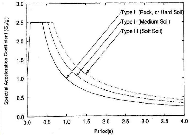
RESPONSE SPECTRA FOR ROCK AND SOIL SITES FOR 5% DAMPING
