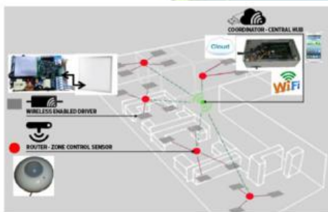
Fig. 1. Typical application scenario of Smart Lighting with the topologies of devices used: i) Coordinator of network connected to a host device; ii) Router to monitor the environment with light and motion sensors; and End Device connected to the panel to adapt the light intensity to save energy achieving the optimal level of brightness in the area.
