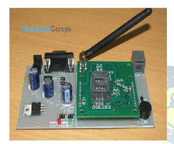
GSM/GPRS MODEM is a class of wireless MODEM devices that are designed for communication of a computer with the GSM and GPRS network. It requires a SIM (Subscriber Identity Module) card just like mobile phones to activate communication with the network. Also they have IMEI(International Mobile Equipment Identity) number similar to mobile phones for their identification. A GSM/GPRS MODEM can perform the following operations:
