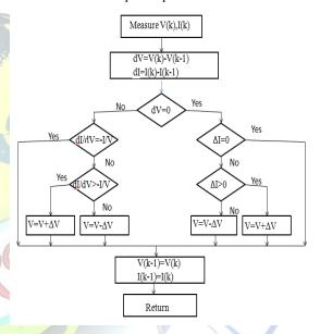
Fig 2 Flowchart of incremental conductance algorithm
