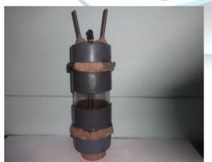
Fig. 1 hydroxy generator
