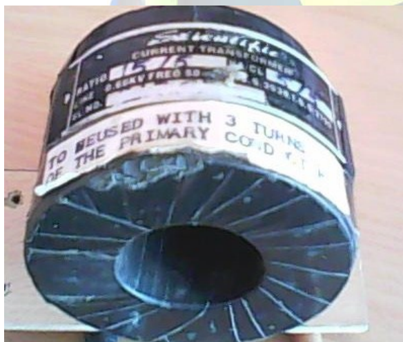
Fig. 2 Current Transformer
