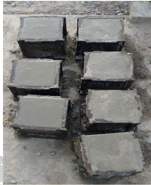
Fig.5 Casting cube specimens
