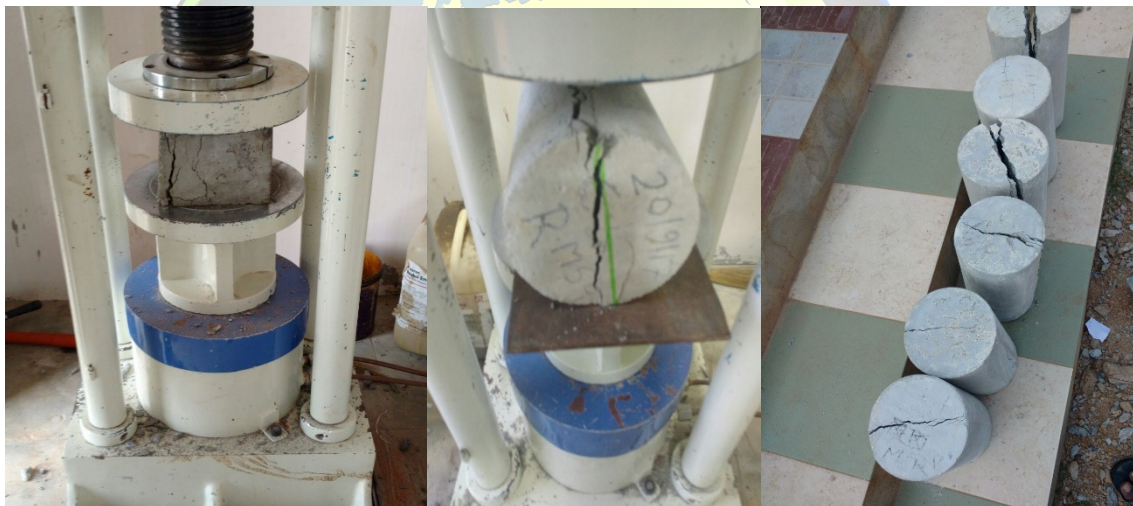
Fig.6 Testing of Concrete cube & cylindrical specimens
