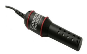
The CO2 Gas Sensor measures gaseous carbon dioxide in two ranges—0 to 10,000 ppm and 0 to 100,000 ppm with this sensor, you can easily monitor changes in CO2 levels occurring in respiration of organisms ranging from peas to humans on the high range, you can explore human respiratory changes in CO2 levels based on exercise.
