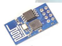
The ESP8266 is a low-cost Wi-Fi microchip with full TCP/IP stack and microcontroller capability produced by Shanghai-based Chinese manufacturer, Espressif Systems. This small module allows microcontrollers to connect to a Wi-Fi network and make simple TCP/IP connections using Hayes-style commands.
