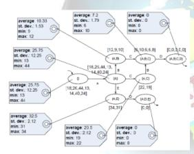
The annotated transition system showing per state: the average, standard deviation, minimum, and maximum remaining time until completion.
