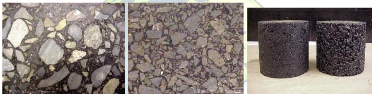
(a) Dense graded asphalt (b) Stone Matrix Asphalt (c) Dense-Graded HMA (left) vs. SMA (right)
