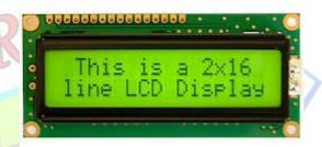
An LCD consists of two glass panels, with the liquid crystal material sand witched in between them. The inner surface of the glass plates are coated with transparent electrodes which define the character, symbols or patterns to be displayed. Polymeric layers are present
